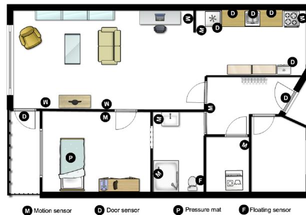
**Figure 1:** A map of the volunteer's apartments equipped with a wireless sensor network. The orientation of the motion sensor is indicated by the orientation of the letter M.
