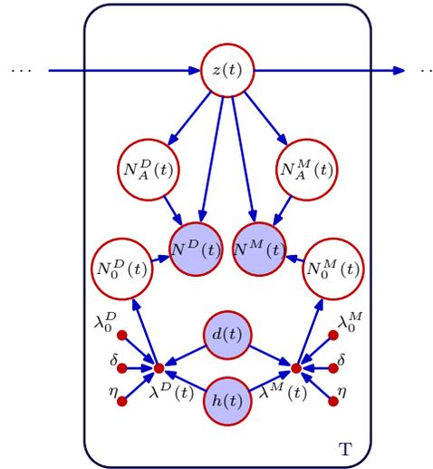
**Figure 2:** Graphical model for different distributions and variables defining the M3P2. The shaded nodes are observed and the small solid nodes indicate deterministic parameters. The directed edges indicate conditional dependence of the nodes.  $\lambda^M(t)$  depends on the parameters  $\lambda_0^M$ ,  $\delta$ ,  $\eta$ ,  $d(t)$  and  $h(t)$ , while  $N^M(t)$  depends on  $N_0^M(t)$ ,  $N_A^M(t)$  and  $z(t)$ .
